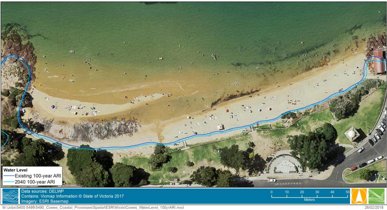
Figure 4-2 Extent of 100-year ARI water levels on the site for present day and 2040
