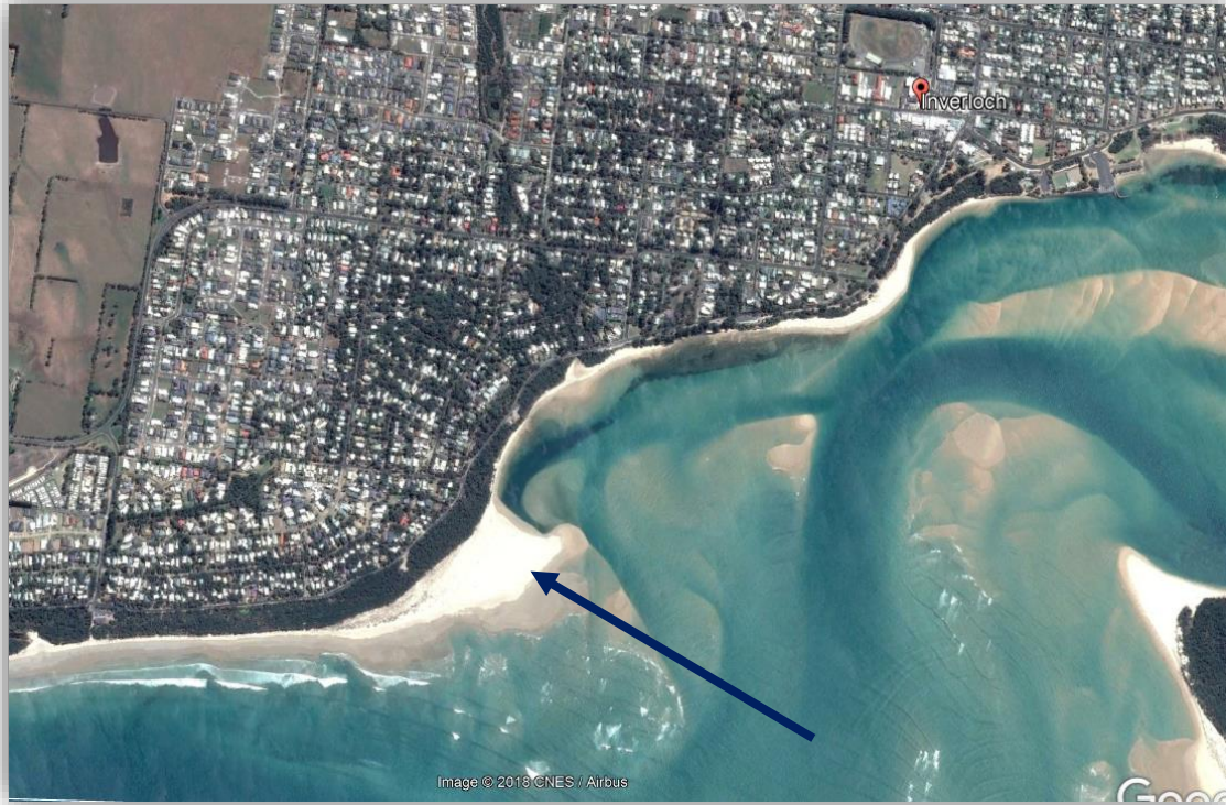
Figure 2 - Satellite image of Ayr Creek in January 2014, showing the spit curving in at Point Norman (identified by the blue arrow), but no lagoon. Note how the sand spit has blocked off the deep entrance channel (Source: Google Earth).
